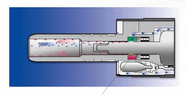
The KaVo Care-Ring protective barrier guards against contamination. All cleaning and care agents are trapped so that they do not reach the inside of the motor. And because the motor is not contaminated, its life is increased.
