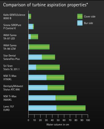
\* Sealed measuring under vacuum during the slowing down phase (measured in cm of water)
