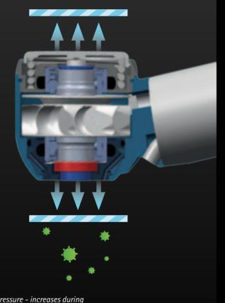
Overpressure - increases during slowing down phase of the cartridge
